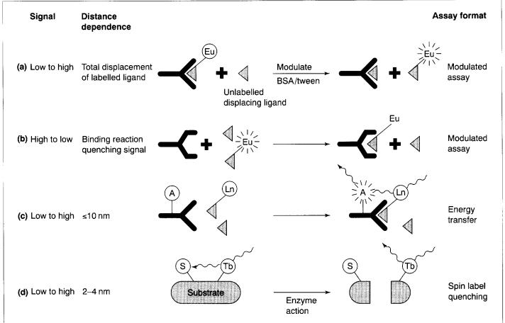
**Figure 2.** Principles of time-resolved fluorometric homogeneous assays based on environmentally sensitive chelate labels or energy transfer. A, acceptor molecule (e.g. tetramethylrhodamine, A-PC or Cy-5); BSA, bovine serum albumin; Eu, europium chelate; Ln, terbium or europium chelate; S, spin label.
